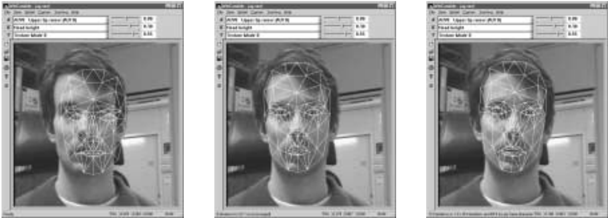
Figure 5. The face model approximately adapted to the face image ( left ); The face model adapted by the Active Model step (after pressing Ctrl+1 twice) ( middle ); After tracking the face through frames 11 - 20 in the test sequence ( right ).
