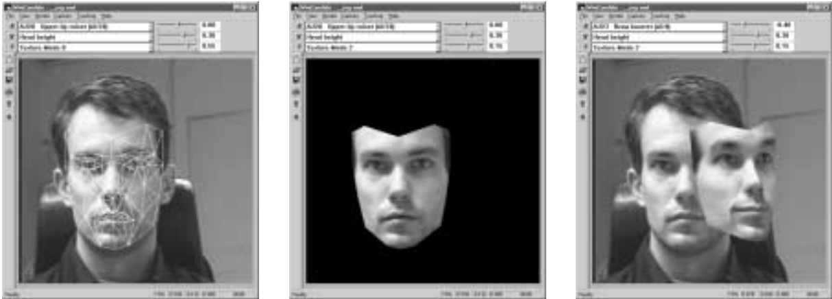
Figure 3. Taking a texture from a background image. Left image: The model has been adapted to the background image. Middle image: The texture has been taken as texture (Ctrl+T) and the background made invisible (Alt+V+B). Right image: The model is moved away from the previous position and modified slightly using the animation units.
